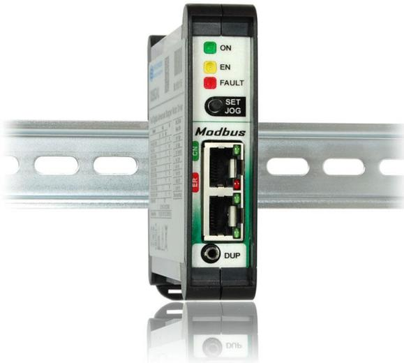
The physical layer is **RS485** type and isolated from the auxiliary and power supply, the communication speed reaches **921.600Kbit/s**. Among the implemented functions is the **23 0x17 Read/Write Multiple registers** which allows in a single transaction to read and write multiple registers at the same time and can be used, for example, to update the position set point and read the encoder quota in a single operation.
