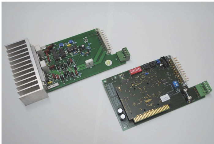
Figure 2: smOOver.opt with plugged in smOOver.drv (front right) compared to original „CNC-Steuerkarte“ (back left).
