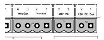
**Slider SFX** can convert a PWM input signal (min. PWM frequency 200 Hz) to an analogue output signal. Many frequency converters accept such a signal as reference value for the rotational speed of synchronous or asynchronous main spindle motors. Consult the manual of your converter to see how the reference input has to be parameterised.
