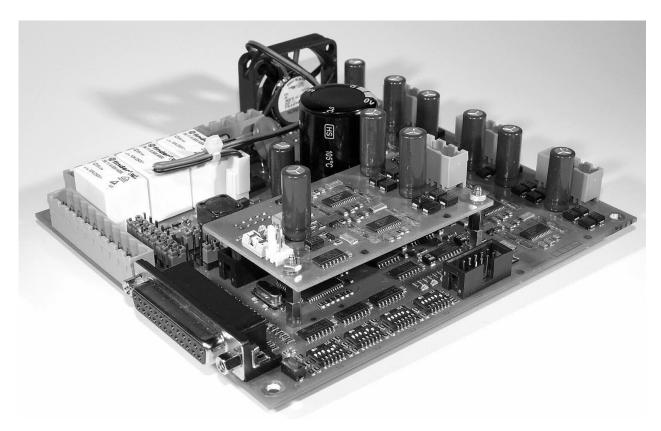
To upgrade **Slider SFX** to a 4 axes driver, connectors X9 and X14 provides the necessary control signals. The upgrade is done with a small add on board, that includes all components including the connector for the 4th motor.
