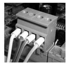
On all connections care should be taken to achieve the best possible contact. All signal and motor wires should be be equipped with core cable ends. To avoid disturbances especially on the switch inputs on X7, shielded and/or twisted pair wires have to be used.
