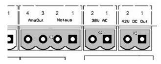
When decelerating, a stepper motor acts as a generator and supplies current back to the power supply. This will temporarily cause the supply voltage to increase significantly. To prevent rising above 45VDC, an electrolytic capacitor can be connected to clamp X5 in addition to the capacitor in the pow-
