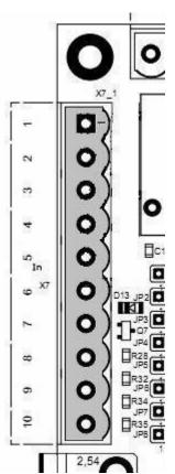
The stepper motor board *Slider SFX* has 5 inputs that are forwarded to signals on the 25 pin D-Sub type connector. These are exactly the signals, which are used as inputs on the PC parallel port. Switches with both N.O. or N.C. can be used. For each input, two cage clamp contacts are present.
