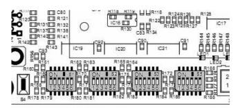
The stepping motor drivers support microstep operation. They produce a sinusoidal course of motor currents. The step width can be set individually for each motor with the left three DIP switches according to the following table.
