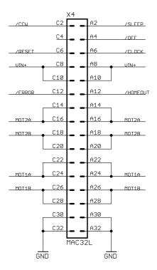
/CCW direction of movement, counterclockwise at low level
