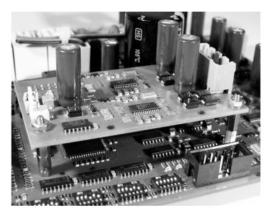
With an addon board, *SliderSFX* is capable of driving 4 axies. The plugin position with two connectors and mounting holes is placed directly abouve the DIP switches.
