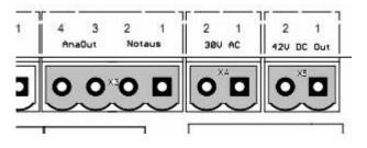
We recommend a transformer or power supply rating of 100VA to 160VA, depending on the employed motors and the voltage level of the supply. We would be happy to give you an advice. To follow the EMC regulations an adequate supply filter has to be used in addition the transformer used in your application.
