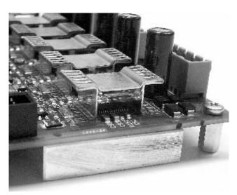
in housings and machines where this maximum temperature is not exceeded. A fan mounted to the side of the board or a case fan ensures proper cooling. A filter with 30 ppi or higher is required.
