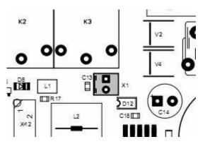
On the connector X1 5VDC are supplied for the fan mounted to the side of the board. This fan can be mounted on the upper or lower side of *Slider SFX*, depending on mounting situation and ventilation in the case. If a case with integrated fan is used, the air stream should pass the 6 drivers (IC's 1, 2, 5, 7, 12 and 17). The direction of the board's fan air stream should be adjusted in the same direction as the case fan. In this case the fan mounted to the board may be redundant.
