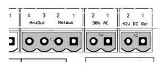
The ready or emergency signal on clamp X3, contacts 1/2, activates the three power drivers for the motors and also acts as enable signal for the relays. The signal is routed to the enable input of the power drivers and can therefore be used as an emergency signal or as a contact of a protection hood.
