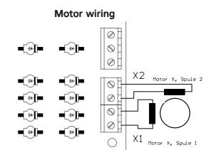
latter may offer a higher rotational speed for which you have to pay the price of a higher current leading to a lower torque when the phase current exceeds 2 amps. Using this arrangement the coil resistance is cut to half and should not fall below 0.8 Ohms. Once you are above that you may try both options.
